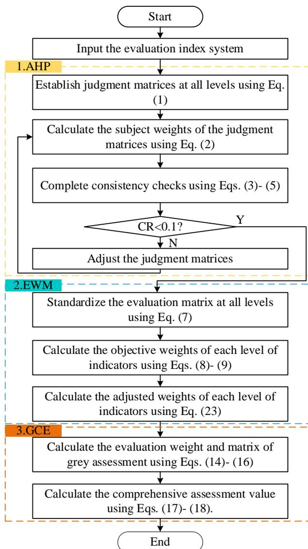
Fig. 3. Evaluation flowchart based on AHP-EWM-GCE.
