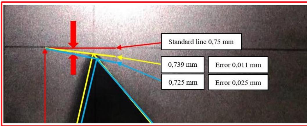
Fig. 12. Comparison of thread height errors before and after polishing at 110 min.
