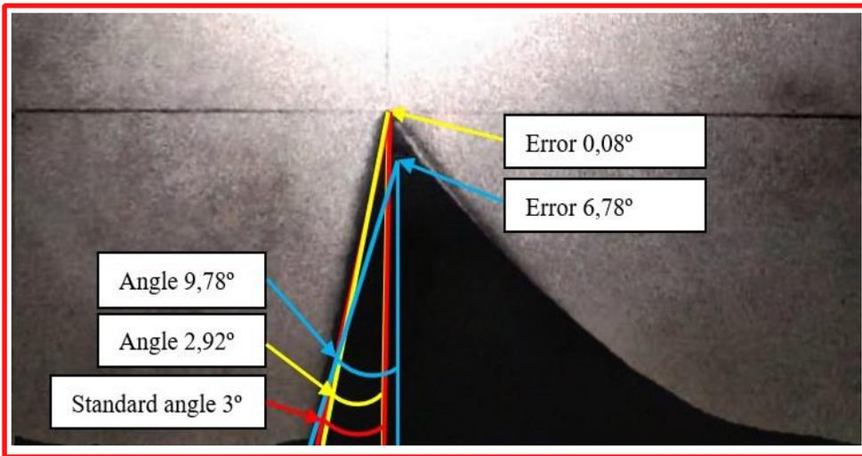
Fig. 18. Comparison of thread angle  $\beta$  errors before and after polishing at (c) 110 min.
