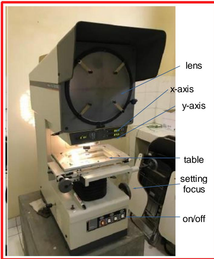
Fig. 3. Profile projector used in this experiment
