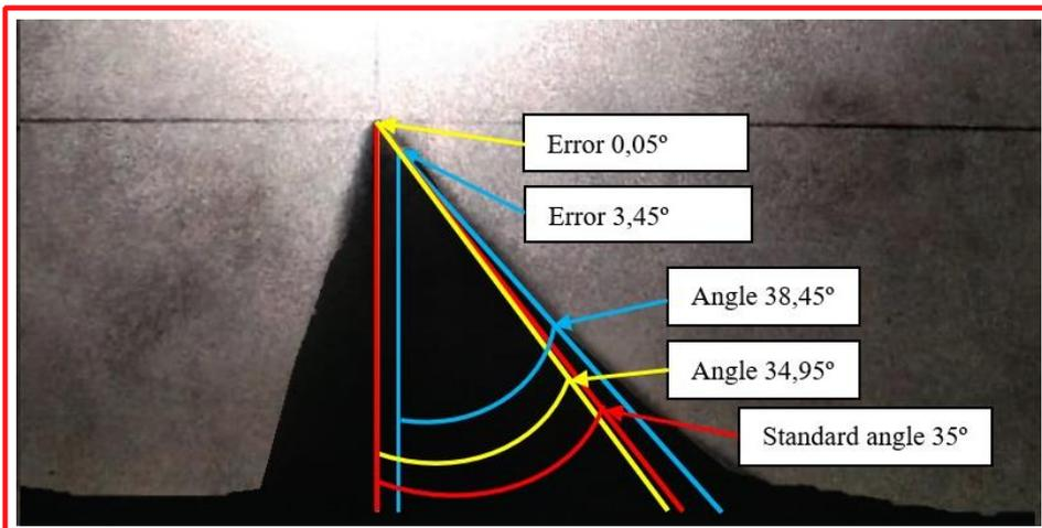
Fig. 15. Comparison of thread angle  $\alpha$  errors before and after polishing at 110 min.
