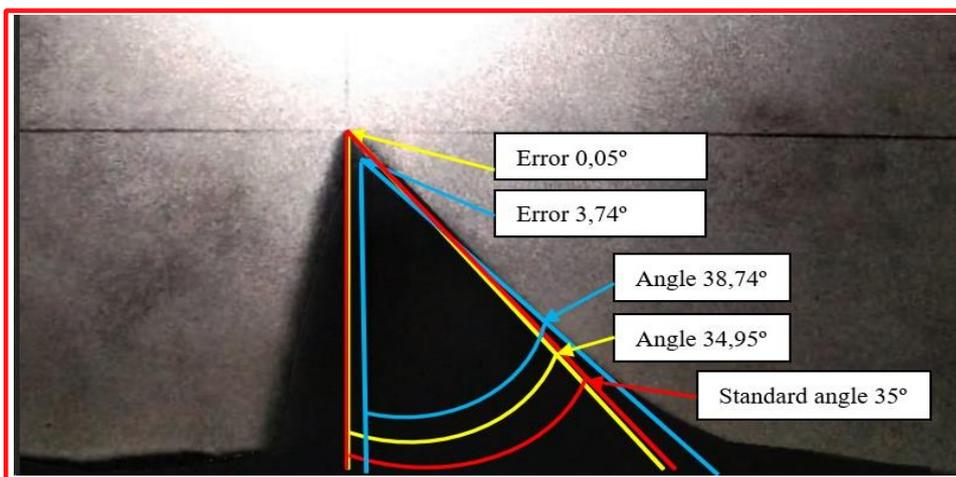
Fig. 14. Comparison of thread angle  $\alpha$  errors before and after polishing at 100 min.
