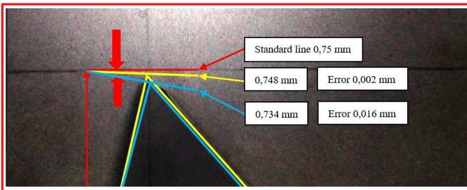
Fig. 10. Comparison of thread height errors before and after polishing at 90 min.
