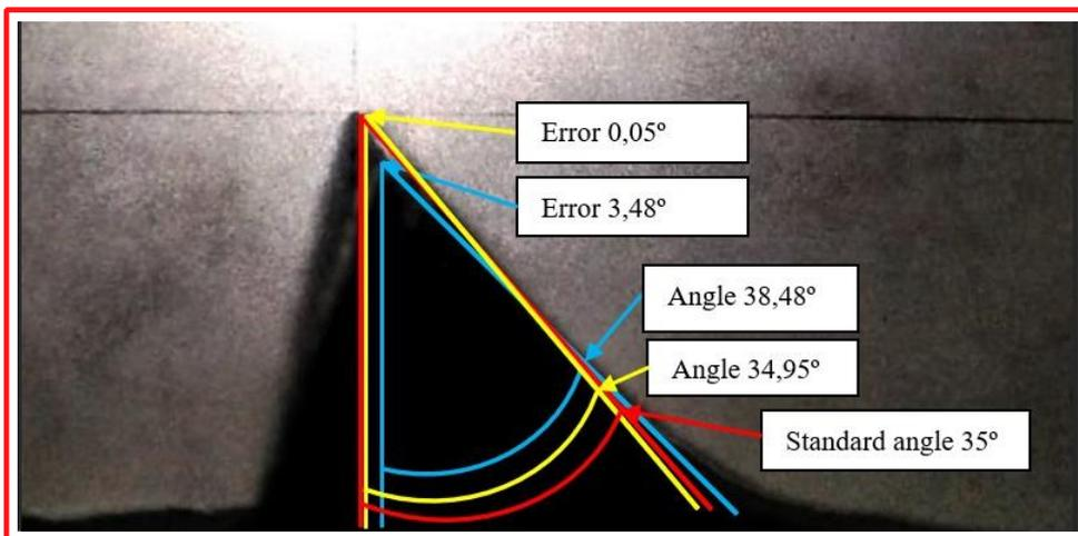
Fig. 13. Comparison of thread angle  $\alpha$  errors before and after polishing at 90 min.
