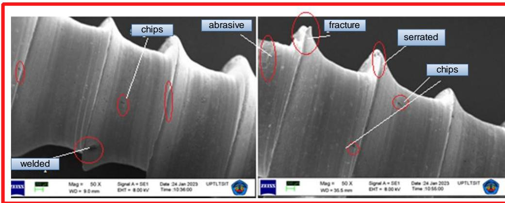
Fig. 19. Surface damages of cortical screws when polishing for 90 min.
