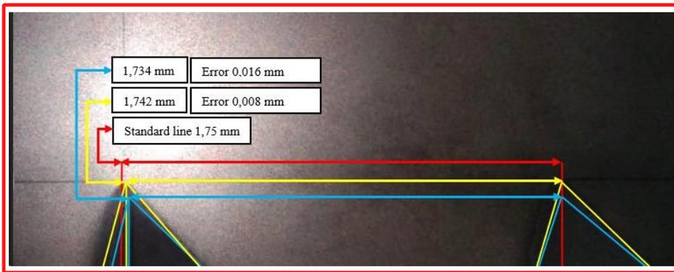
Fig. 8. Comparison of pitch peak distance errors before and after polishing at 100 min.
