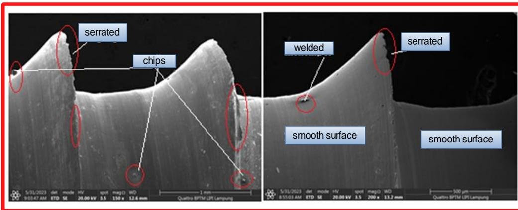
Fig. 20. Some surface damages of cortical screws and the smooth surface of the screw.
