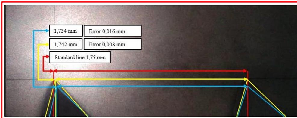
Fig. 9. Comparison of pitch peak distance errors before and after polishing at 110 min.
