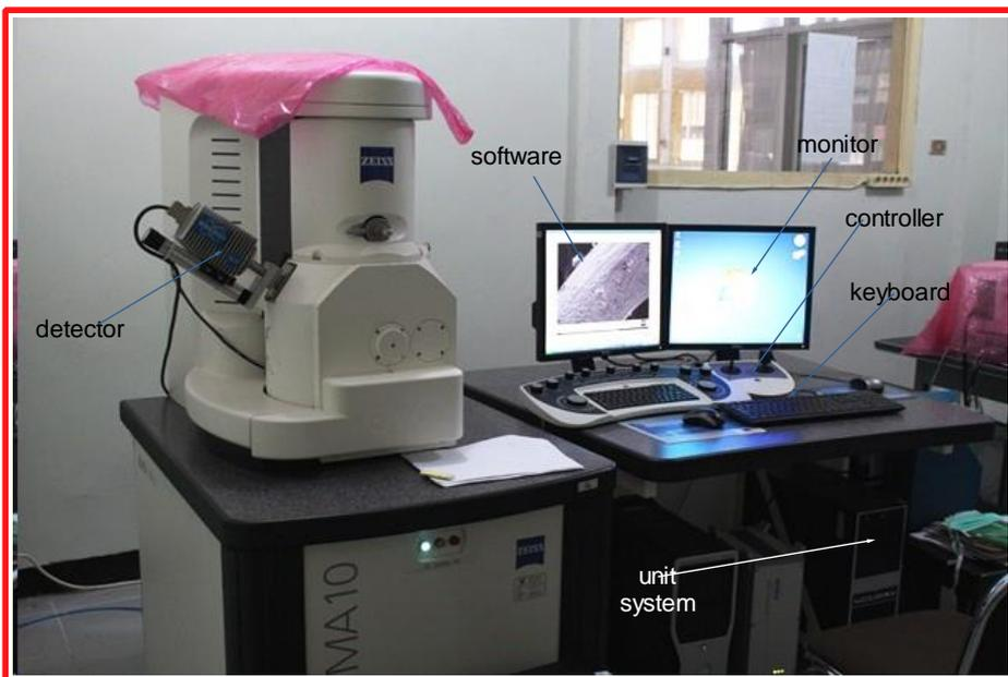
Fig. 4. SEM-EDX Zeiss EVO MA 10 for identifying dimension errors
