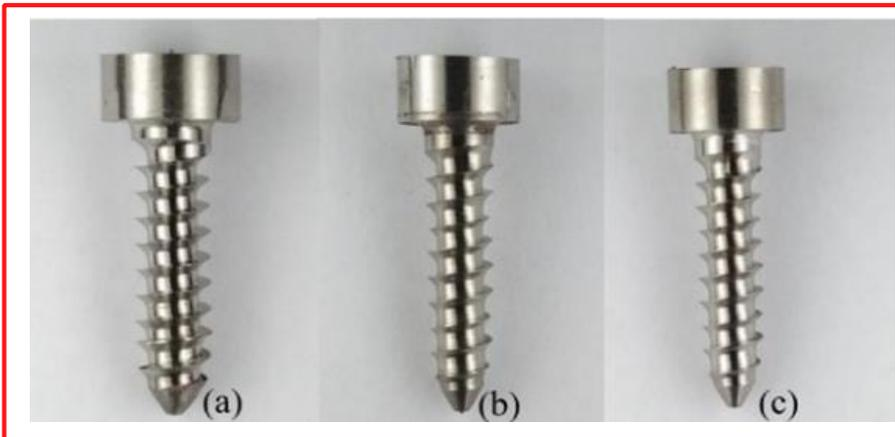
Fig. 6. Polished screw for (a) 90 min, (b) 100 min, and (c) 110 min.
