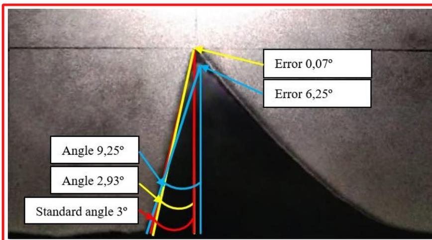
Fig. 17. Comparison of thread angle  $\beta$  errors before and after polishing at (b) 100 min.
