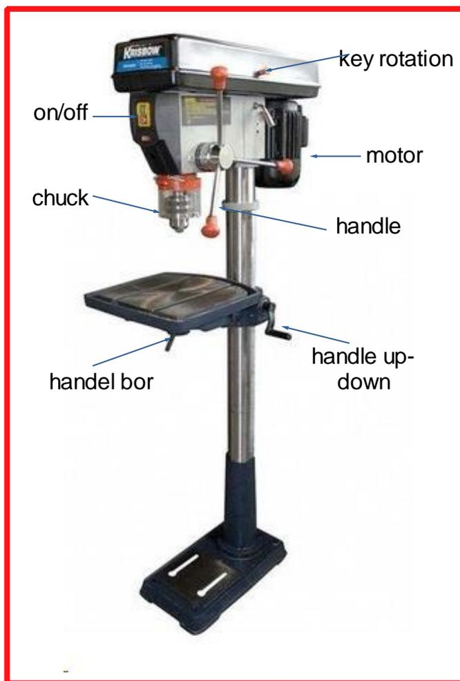
Fig. 2. KRISBOW 16 mm drilling machine
