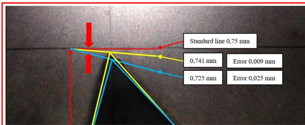
Fig. 11. Comparison of thread height errors before and after polishing at 100 min
