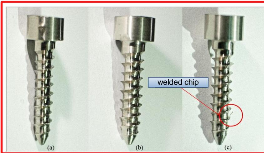
Fig. 5. Threaded screw cortical before the polishing process
