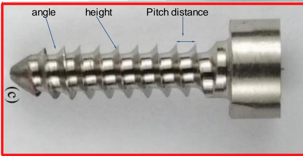
Fig. 1. Cortical threaded bolt (Ti-6Al-4V ELI)
