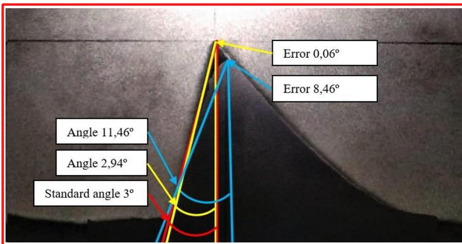
Fig. 16. Comparison of thread angle  $\beta$  errors before and after polishing at (a) 90 min.
