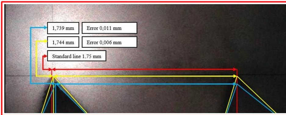
Fig. 7. Comparison of pitch peak distance errors before and after polishing at 90 min.
