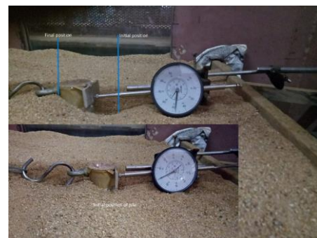
Fig. 5. Initial and final position of pile head
