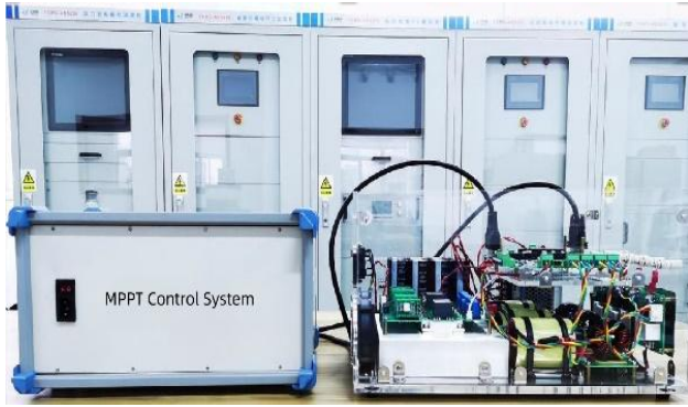
Fig. 9. Photovoltaic MPPT control experimental platform
