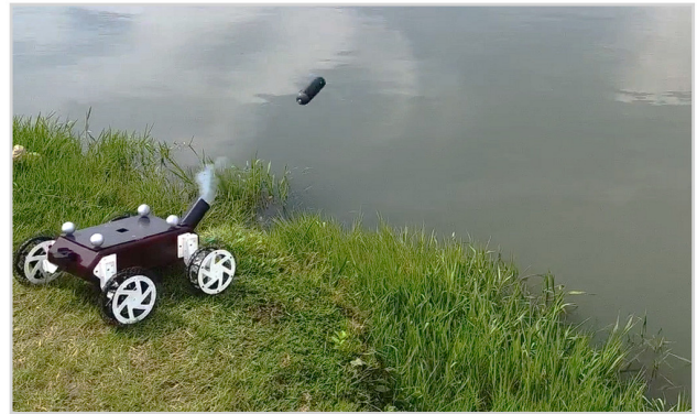
Fig. 1. The ground robot with a sensing device and launching and retrieval mechanisms designed for crater lake geochemical monitoring.
