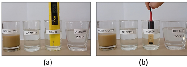
Fig. 16. The data gathering procedure using pH meter (a) and pH sensor (b) for three liquids: liquid A (matcha latte), liquid B (tap water), and liquid C (bleach).
