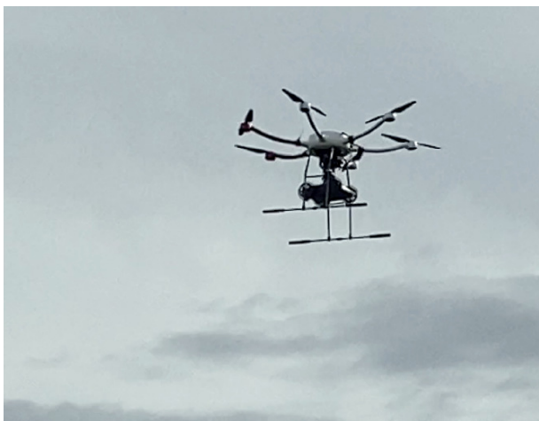
Fig. 3. An example of actual deployment operation of the ground robot utilizing a high payload drone. The drone carrying the ground robot will transport the ground robot to the area of deployment.
