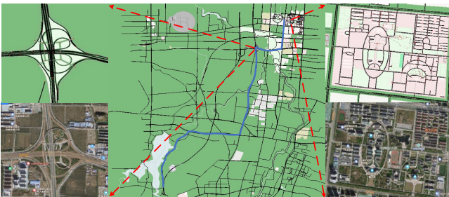
Fig.3. Road network model and actual satellite comparison
