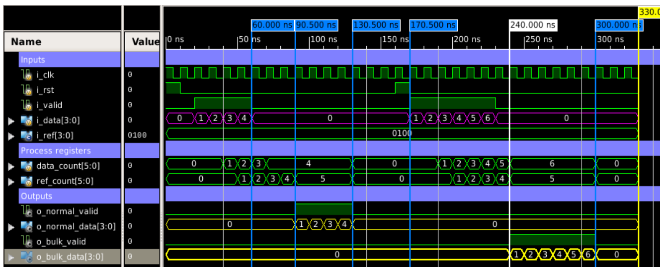
Fig. 17. Simulation waveform depicting data segregation as normal and bulk data by DSIR
