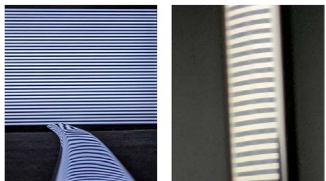
Fig. 5 (Left) Image taken with the camera’s viewpoint set to “just above the surface.” At the back is a stripe-pattern light source. (Right) Image of the same object when the angle between the camera’s line of sight and the normal is set to almost zero.
